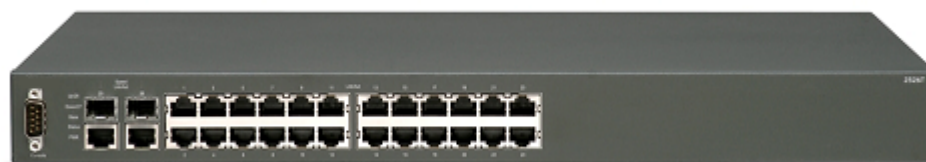
Figure 27: TLAN Layer 2 switch (Ethernet Routing Switch 2526T)
